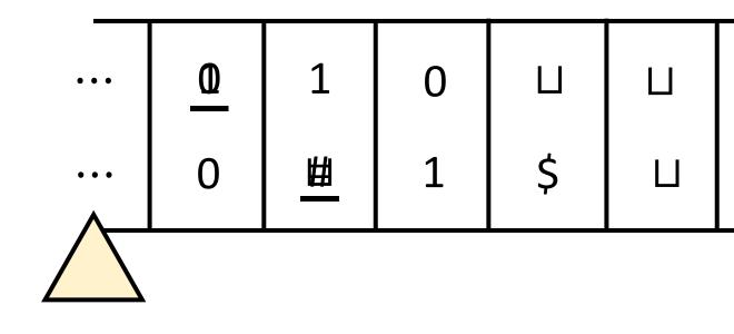
• The one "real head" will scan back and forth, updating the simulated heads' locations and the simulated tape contents. (Details on the next slides)
